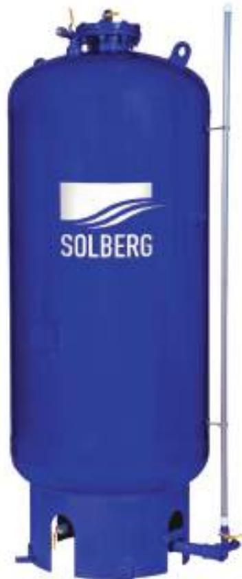
out of SA 516 Grade 70 carbon steel with a nylon reinforced neoprene rubber bladder. It has a perforated center tube, and a .37" (9 mm) water channel between the water inlet and water drain valve, which creates a water path between the bladder and tank shell. Openings that are greater than 1.0" (25 mm) will be divided to prevent bladder damage.
